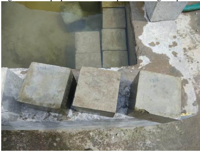
Fig. Shows the compressive samples of concrete
