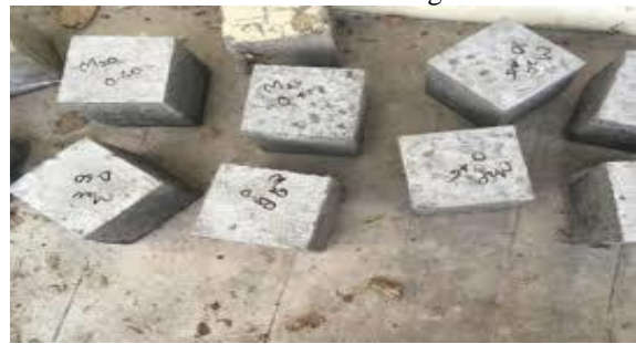
Fig.4.15Shows the compressive samples of silica fume-concrete
