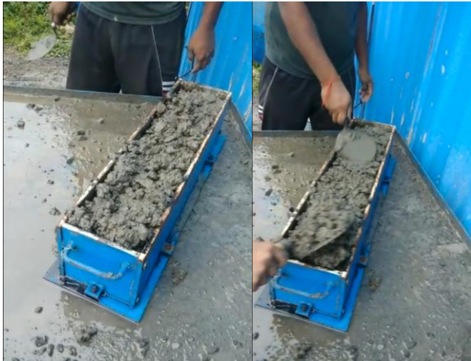
Fig. shows the preparation of three-point bending samples
