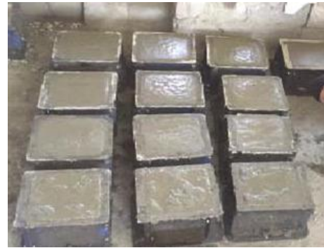
Fig. compressive samples of fly ash-silica fume concrete
