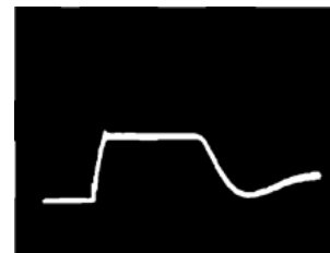
Figure 10. Starting response of armature current: experimental result for 1-P control
