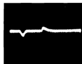
Figure 17. Response to a load disturbance for P-I control: experimental result.
