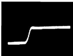
Figure 13. Response to a change in speed reference for J-P control: experimental result.
