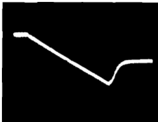
Figure 19. Speed response for a reduction in speed reference command.
