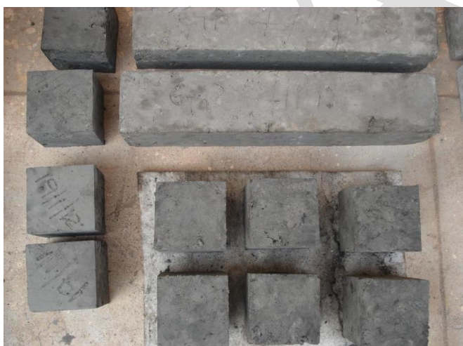
Fig. shows the compressive and flexural samples prepared from fly ash and silica fume mixture concrete
